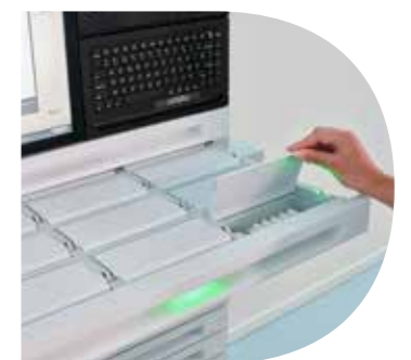
Smart Cart assigns a medication bin for each patient, opens bin for nurse to place all medications
